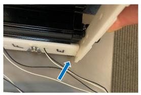
**Step 4)** Route the reed switch wires through the service port in the front of the machine and around to the circuit board. (Shown Below)
