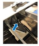
**Step 1)** Remove the top by following the top removal instructions. Measure the locations of the three switches. Measure from the end of the actuator rail to the far ends of the reeds. Then loosen allen bolts on the three reed switches and slide them off of the main actuator rail starting with the blue sensor.
