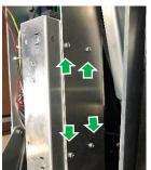
**Step 3)** Remove high voltage and low voltage wires from power supply. Then remove the 4 phillips screws holding the power supply to the machine. Right angle screw driver attachment is very helpful.
