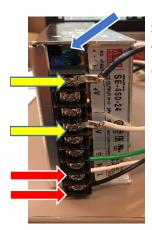
**Step 5)** Reapply power to the machine. Check output voltage. Verify that it is set at 24V +/- .5V. Use adjustment screw to set voltage correctly. Verify that the power supply input voltage is set to 110V on
