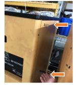
Step 1) Remove compactor top and front door skin. (Refer to ISO001 and ISO002) If only adjusting the L-Bracket, remove only the front door skin and refer to step 5.
