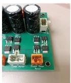
**Step 2)** Remove Trash Door Motor terminal block from circuit board and remove the wires from the terminal block and route wires back to trash door actuator
