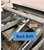
Step 4) Remove the two main actuator bolts starting with the back bolt. Start by adjusting jack height to reduce the weight on the actuator bolts. Once you have removed the back bolt, restore power to the machine. Jog the actuator up by referring to Step 2 and pressing increase to move the head up to a workable position: for easier removal.
