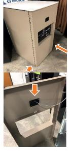
**Step 2)** Using a T-25 torx wrench remove the three screws located on each side of the front door skin. Pull top of skin forward and lift up and off of bottom tabs.
