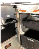
Step 4) Remove three T-25 torx screws from front side and one from bottom left side of both side panels and two T-25 torx screws from back side top of side panels. Remove both rear bumpers using a 5/16 (8mm) nut driver or socket. You are now ready to remove the sides. Note: You may find 4 phillips head screws in the front side and 4 in the back of side skins. Remove these and discard.
