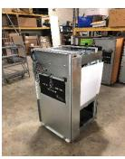
**Step 5)** First install new side skins by reversing previous instructions. Then reinstall LCD into new door Skin. Now install new door skin by placing the bottom of the door skin into tabs that are located at the bottom of the frame and slide top into place. Install door skin screws and reinstall compactor top. Restore power and test LCD function.
