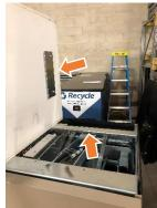
**Step 3)** When reinstalling top, line up the bracket attached to the top and place it into the guides in the frame. Slide the top towards the front of the compactor and line up bolt holes on inside of compactor shown in photos from step above. Tighten bolts.
